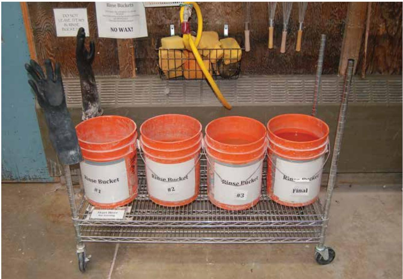
This four-bucket system at the University of Oregon is designed for capturing all glaze waste, which is then used, along with recycled clay, to make paver bricks.
