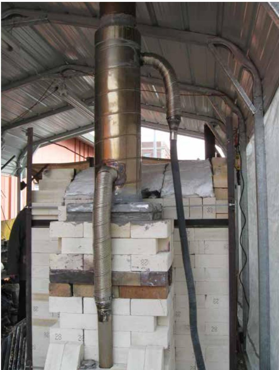
The recuperative chimney on one of Shippensburg University's kilns reclaims heat from the exterior of the chimney and the warm air is used with the drip plate burner system to enhance fuel combustion.
