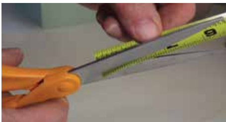
A steel measuring tape is easily cut into thin strips with scissors.
