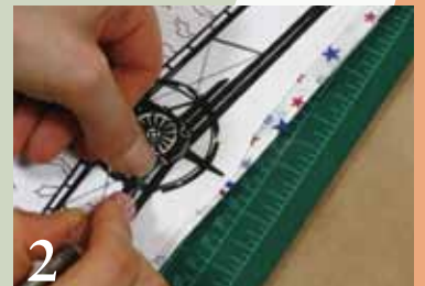
2 Cut interior sections of the stencil first. Compress delicate areas to keep plastic from shifting.
