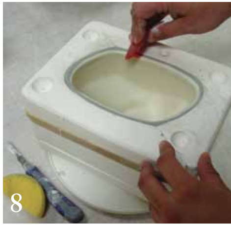
8 Finish the rim with a red rubber rib. Note the striations of contrasting colored slip.
