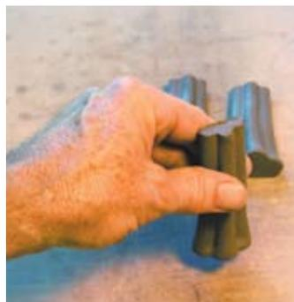
One end of the handle blank is repeatedly pounded onto the table to thicken it. This will become the top of the handle.
