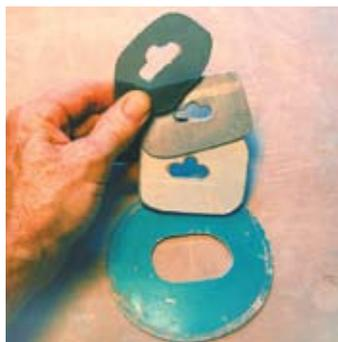
Handle dies in three sizes, for small cups, mugs, and pitchers. Made from aluminum (recycled highway signs) or Plexiglas™ cast acrylic scraps. The shapes were made using a drill and a jeweler's saw. The small dies fit over the opening of the green "donut die" so a new die blank is not needed for each small die.
