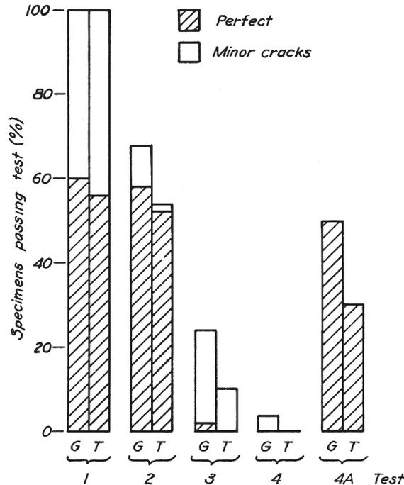
FIG. 3.—Comparison of glaze and terra sigillata.
