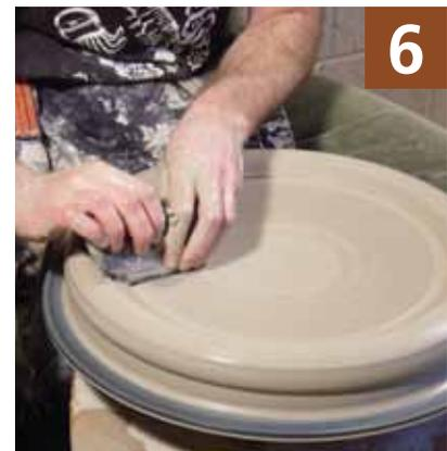
It's relatively easy to throw a large plate (up to 15 inches) from a single ball of clay. When making plates, it's advisable to use clay that is slightly wetter than when throwing vertically oriented pieces. First, wedge a large bit of clay (6-8 lbs.), taking care to eliminate any air pockets that may be present.
