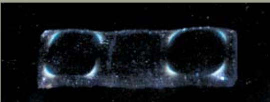
The same glass between polarized film and viewed on a light table. The halos around the Spectrum squares indicate stress due to lack of compatibility. The Bullseye square in the middle has no halo as its COE is compatible with the base glass.
