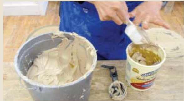
Add stain paste base to the colorant, 3½ parts paste to 1 part colorant by volume.
