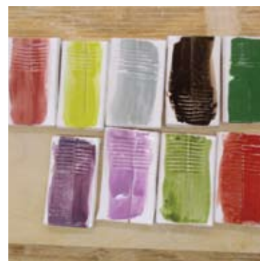
Test tiles of stain pastes painted over majolica glaze and glaze fired to cone 05.
