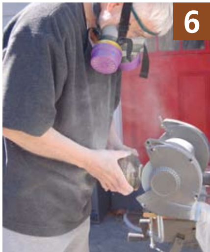
6 Excess pedestal material and glaze are ground off the bottom using a bench grinder fitted with a silicon carbide grinding wheel.
