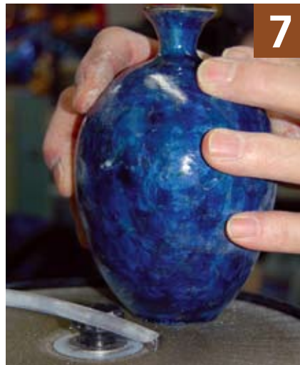
7 I use a portable flat lap machine fitted with diamond grinding and smoothing disks to even out and smooth the bottom of the foot with 100 and 260 grit disks. Since water is used in this process, I do this in the studio, but still wear eye protection. Self-adhesive diamond disks or silicon carbide disks can be attached to plastic bats and the potters wheel used to grind and smooth the bottoms.
