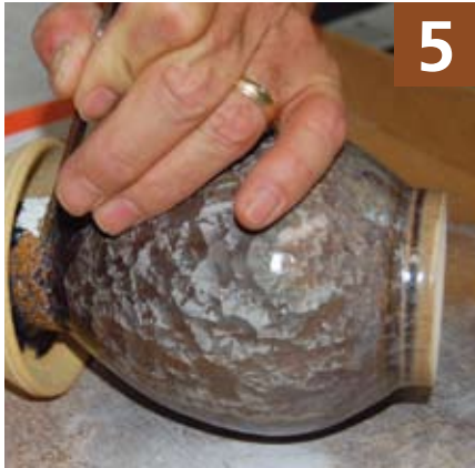
5 The pedestal and catch basin are removed by tapping with a small chisel along the line where the pedestal joins the pot.
