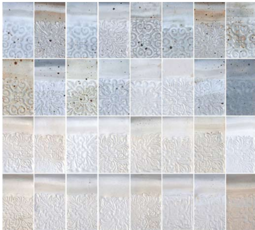
Altering a glaze: The top two rows above were fired to cone 10 reduction in a gas kiln and the bottom two rows were fired to cone 6 electric. Rows 1 and 3 contain 100 extra grams of the tested ingredient listed below each row, and rows 2 and 4 contain none of the tested ingredient.
