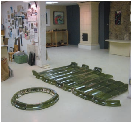
The kacheln laid out in the foreground are for the kachelofen pictured to the right.
