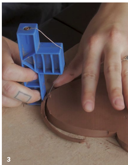
Bevel the edges with the long side of a bevel cutter to create a 60-degree cut.
