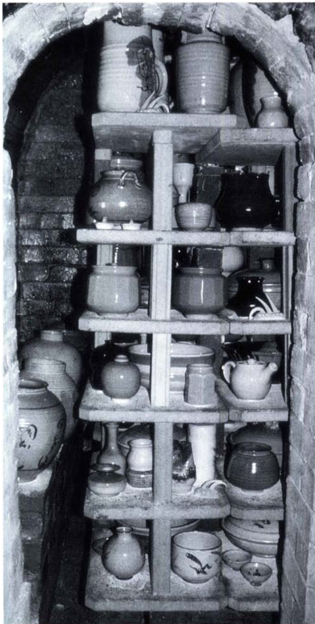
View of third chamber during unloading, showing shelf configuration and pots on bag wall.
