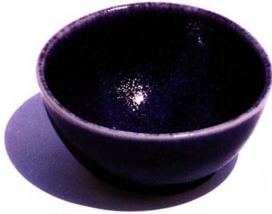
A purple glaze with blue flecks was obtained by adding 3.5% Color Mixture 3 to Copper Red Base Glaze 7.
