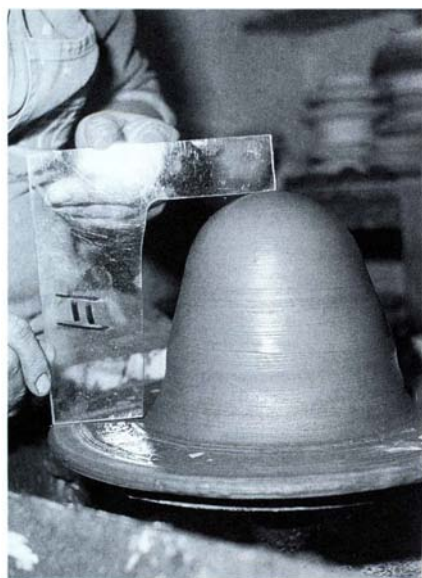
To reconstruct around a solid core, pugged clay is centered on the wheel to a rough height and diameter.
