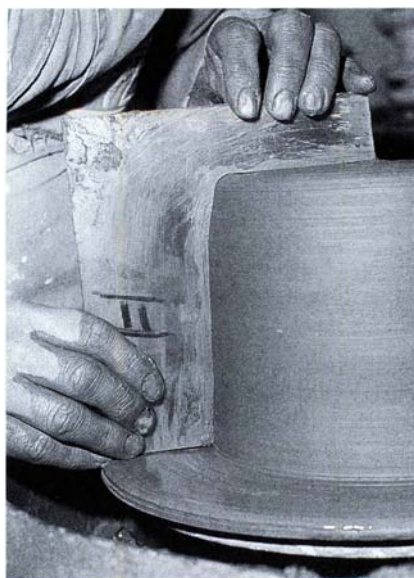
A handheld template is then used to shape the core to correspond with the upside-down vessel's interior.
