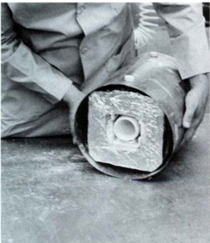
5. Once the assembly is inserted into its metal jacket, the element leads are passed through ceramic insulators set in holes in the jacket.
