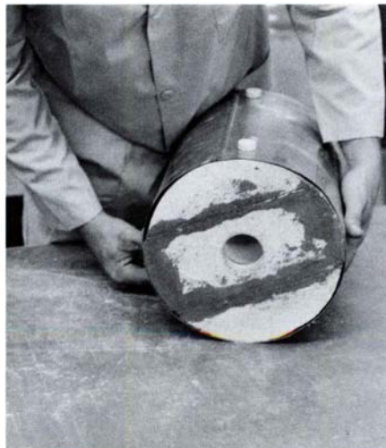
6. Splits from two insulating bricks are cut, shaped and cemented to form end covers for the furnace. A recessed hole supports the refractory tube.
