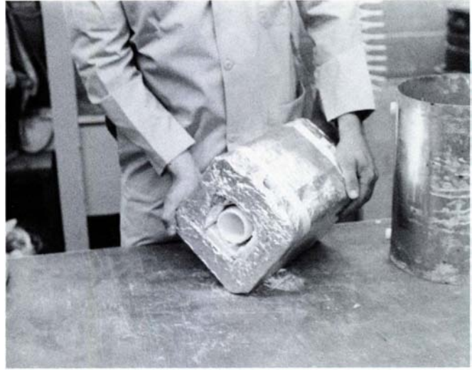
4. The tube, elements and softbrick assembly are bound securely together for ease in inserting it into its jacket, the 12-inch diameter metal drum on the right.
