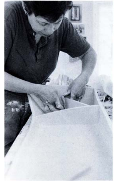
Niches were slab built; coils reinforced the joins.
