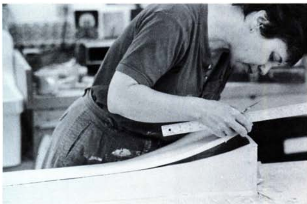
Closing in the left section; after the slab was securely joined, the niche opening was cut out.
