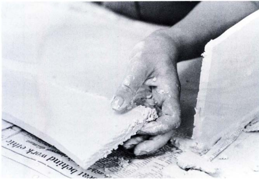
Porcelain slabs (cut to the size of their corresponding cardboard templates) were scored and brushed with slip along the edges, then joined.
