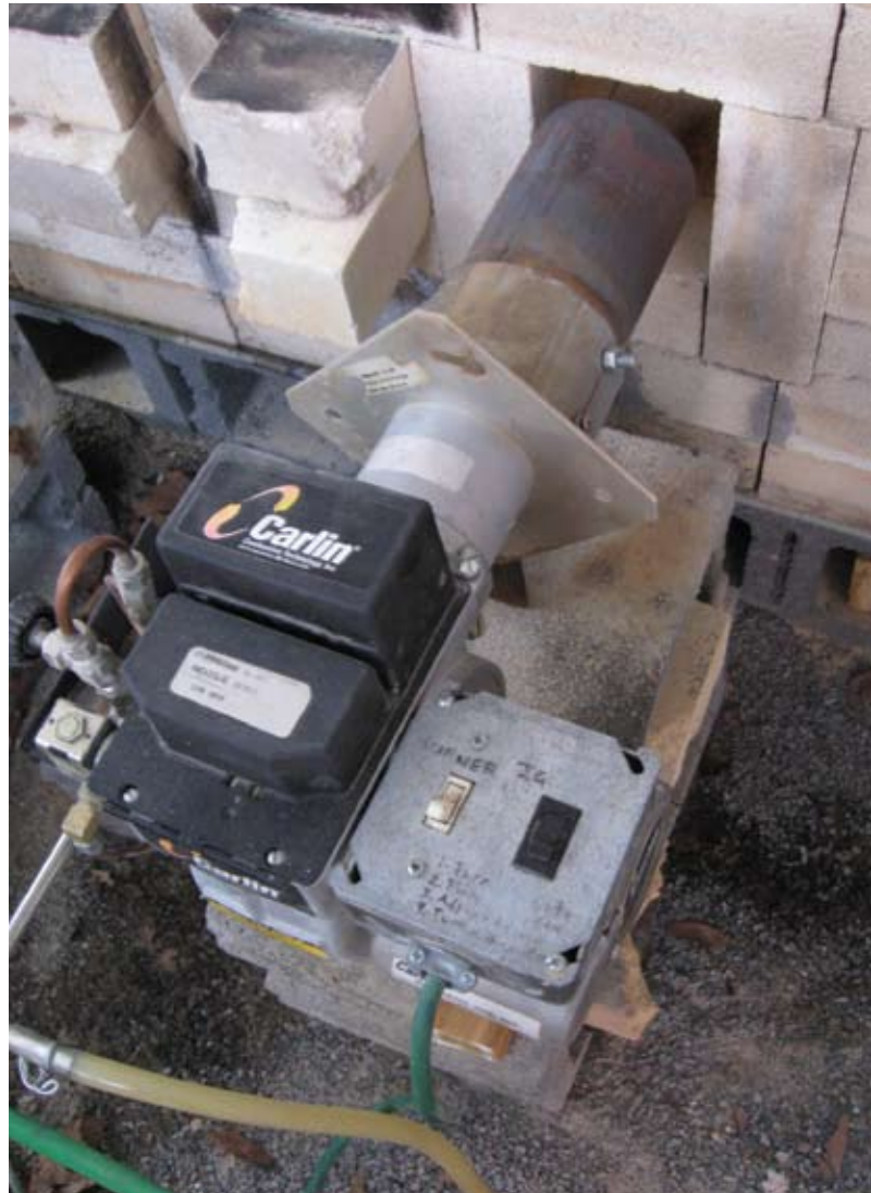
The biodiesel burner and blast tube for vegetable fuel kiln at Shippensburg University (see diagram to the right).
