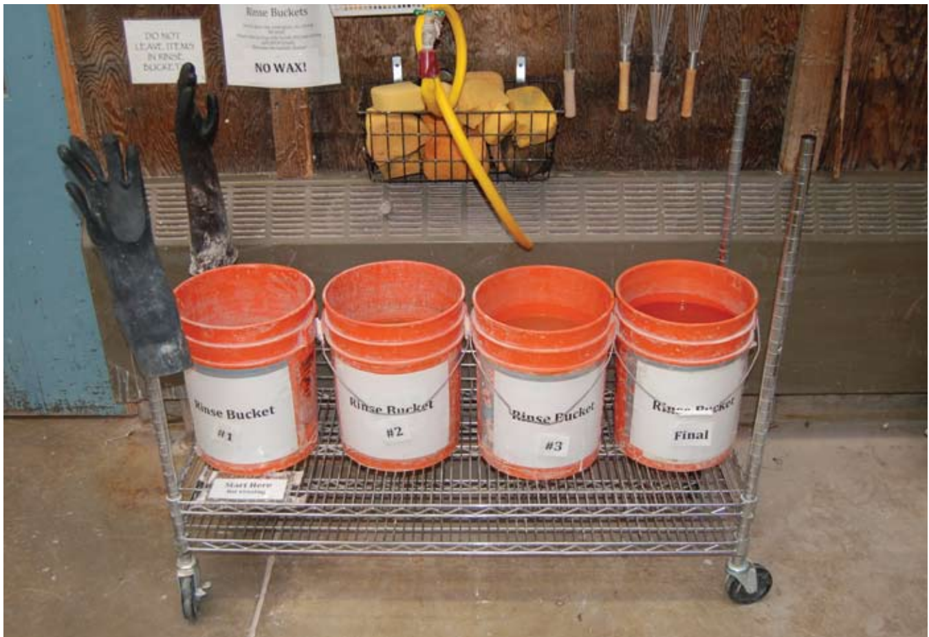
This four-bucket system at the University of Oregon is designed for capturing all glaze waste, which is then used, along with recycled clay, to make paver bricks.
