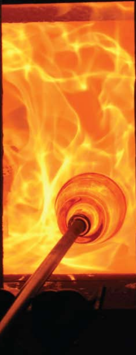
Left: A crucible filled with molten glass at the back of the kiln makes it possible to blow glass while the kiln is being fired. Above: A glass bowl is reheated through the same door opening. Above Right: Steve Gibbs and CCC student Cecilia Charlton stoke the firebox. The air ports below the stoke door lead into the step-grate firebox.
