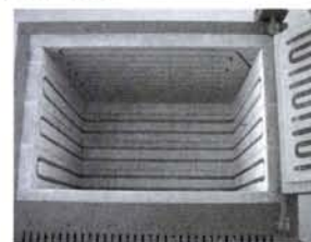
The Janus-24 has elements in the top, sides, back, and door. The top elements use the new pinless firebrick groove.
