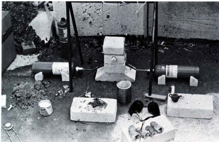
Price-winning miniature kiln fired with propane torches
