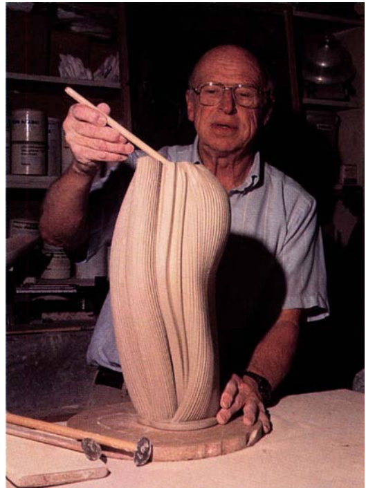
A stick with a metal rib attached to the end is ideal for shaping and refining from the inside of a tall extrusion.
