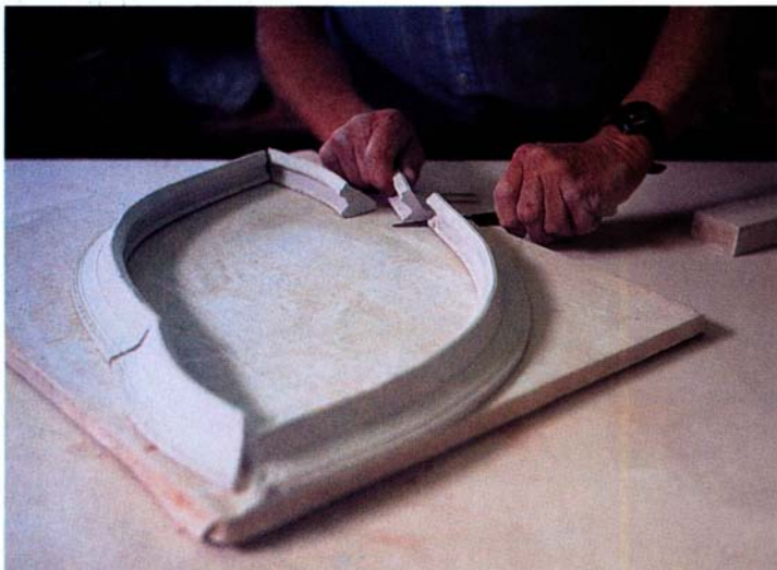
Extruded ridges can be shaped to form the edge of a hump mold. After a bisque firing, they will be glued into position, and the space filled with plaster to complete the mold.
