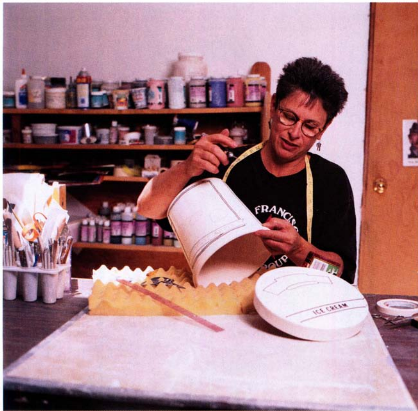
After the initial bisque firing, Shapiro applies surface detail by brushing or spraying underglazes over graphic tape, contact paper cutouts, latex and other resist materials, then fires to Cone 06. The final step for each piece is the firing of a crackle glaze and postfiring reduction.
