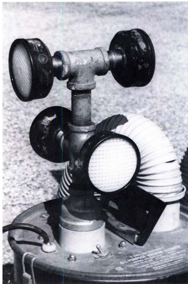
Attached to the blower port with duct tape, the manifold is assembled from 3/4-inch-diameter pipe and organic spray-mask filters (the two have compatible threads). At least two more filters should be added to the manifold for a larger vacuum.
