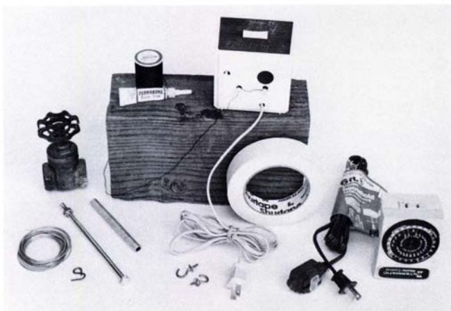
Materials needed to build the timer include tape, hooks, thread and an electric alarm clock with two rotating knobs.
