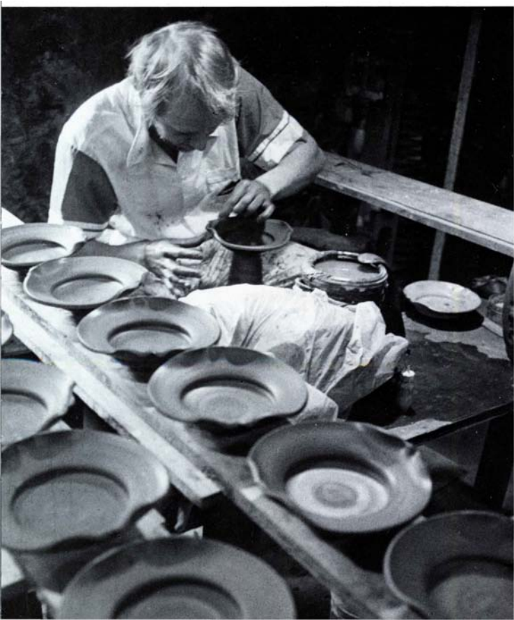
Above and left Richard Bresnahan throws "butterfly dishes" off the hump. From a glacial ridge about 5 miles from his Collegeville, Minnesota studio, he has stockpiled nearly 1800 tons of clay.
