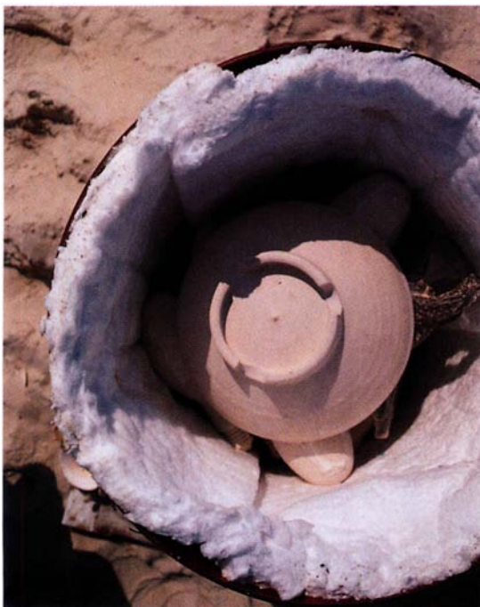
After the refractory blanket was attached and the chamber positioned on the kiln shelf, it was tumblestacked with bisqueware.
