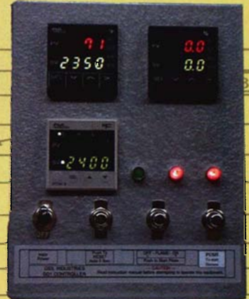
Microprocessors on the kiln control both temperature (ramp/soak) and atmosphere.
