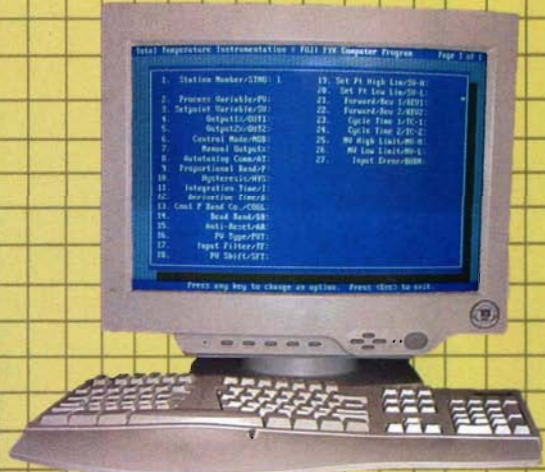
All functions are controlled and monitored from the PC or the kiln.
