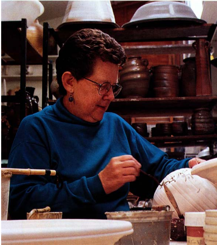
North Carolina potter Cynthia Bringle brushing oxide decoration on bisqueware in her Penland studio.
