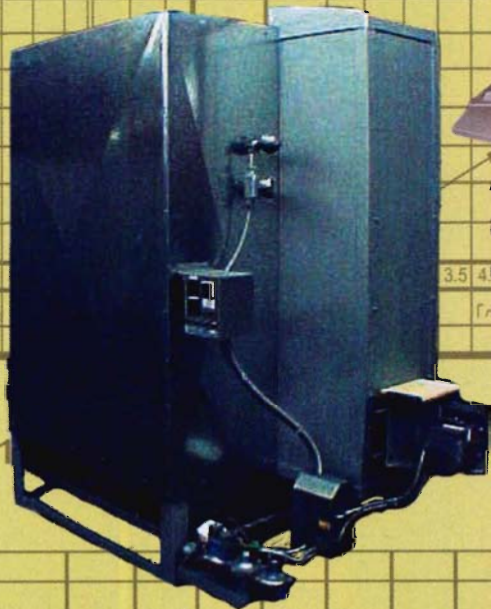
The oxygen probe on the kiln sends atmosphere conditions to the control panel, the microprocessor reads the signal and adjust the damper automatically.
