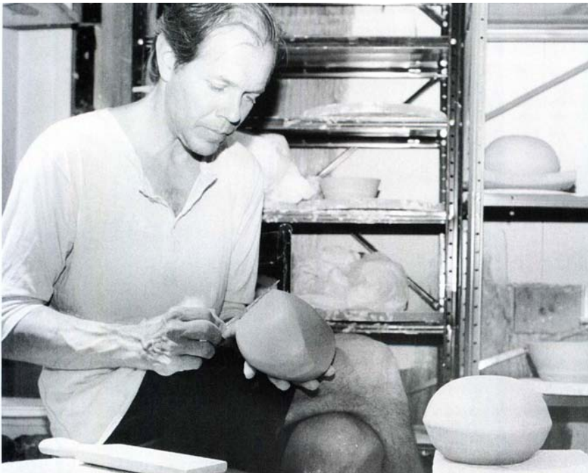
Then edges are accentuated and further defined using a fettling knife,
