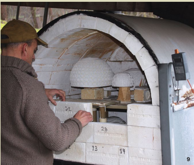
5, 6 HardWired , in progress, adding colored porcelain and using a handmade wooden tool to model the clay straight on the balloon following the lines drawn on the surface. Photos: Katrien Hautekiet. 7 Support for each piece made from porcelain, stoneware clay, and bricks, so that the bowl can be fired upside down. 8 With a small pencil, add porcelain to fix any small holes. 9 Bricking up the kiln door after all the pieces are loaded in the kiln upside down on their firing supports. 10 The door is bricked up, and the firing begins by adding wood to the firebox. 7-10 Photos: Stef Van Leemput.
