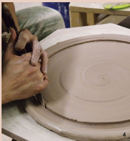
1 Position clay on the bat. 2 Make the bottom of Onggi by using the paddling tool ( Bang-Mang-Yi ). 3 Even out the base by using the paddling tool. 4 Cut off the extra clay to adjust the diameter of the bottom. 5 Attach the first slab to the bottom, forming the wall. 6 Add a coil to join the wall and bottom.
