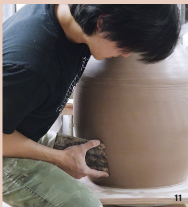
7 Center and smooth the surface using wooden ribs. 8 Attach the next slab and repeat the process. 9 Center and adjust using wooden rib tools. 10 Even the thickness of the wall by using paddling Onggi tools (Surae, outside padding tool, and Dogae, inside padding tool, shown here). 11 Form the Onggi shape by stretching the wall using wooden rib tools. 12 Water storage Onggi, 13 in. (33 cm) in diameter, iron-rich clay, wood and salt fired to cone 9–10, reduction cooled, 2018. All process photos: Rachelle Le Roy .
