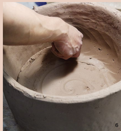
1 Position clay on the bat. 2 Make the bottom of Onggi by using the paddling tool ( Bang-Mang-Yi ). 3 Even out the base by using the paddling tool. 4 Cut off the extra clay to adjust the diameter of the bottom. 5 Attach the first slab to the bottom, forming the wall. 6 Add a coil to join the wall and bottom.
