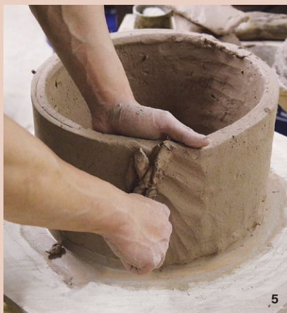
1 Position clay on the bat. 2 Make the bottom of Onggi by using the paddling tool ( Bang-Mang-Yi ). 3 Even out the base by using the paddling tool. 4 Cut off the extra clay to adjust the diameter of the bottom. 5 Attach the first slab to the bottom, forming the wall. 6 Add a coil to join the wall and bottom.
