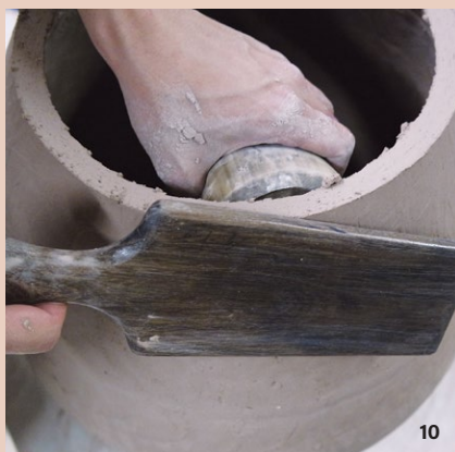
7 Center and smooth the surface using wooden ribs. 8 Attach the next slab and repeat the process. 9 Center and adjust using wooden rib tools. 10 Even the thickness of the wall by using paddling Onggi tools (Surae, outside padding tool, and Dogae, inside padding tool, shown here). 11 Form the Onggi shape by stretching the wall using wooden rib tools. 12 Water storage Onggi, 13 in. (33 cm) in diameter, iron-rich clay, wood and salt fired to cone 9–10, reduction cooled, 2018. All process photos: Rachelle Le Roy .
