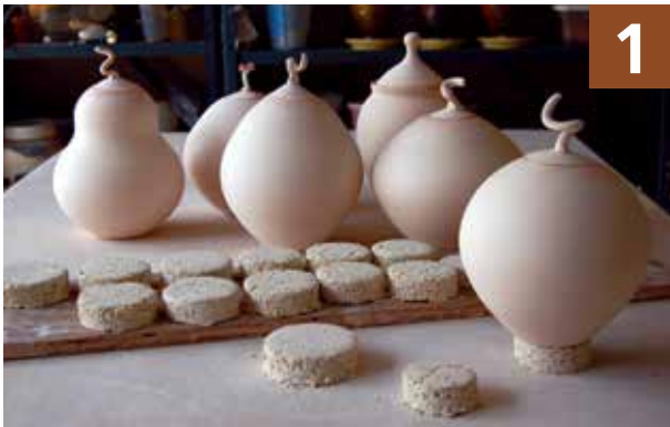
Crystalline glazes run off the pot so you need to raise the piece on a pedestal that sits in a catch basin. It's important to select a pedestal that closely matches the diameter of the foot. Preparing several sizes allows you to select one with the correct fit.
