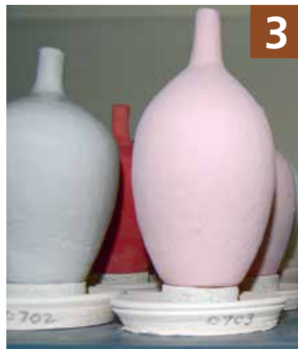
Pieces ready to load in the kiln. Each glazed pot is positioned on a pedestal that is placed in a catch basin.
