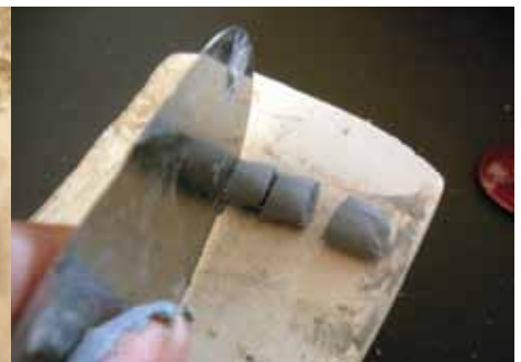
Cut the paste into small objects or beads using a thin metal rib.
