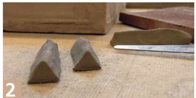
2 Prepare triangular stilts to support the bars.
