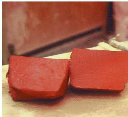
Stack-and-slam wedge 20 times: 1,048,576 layers.
