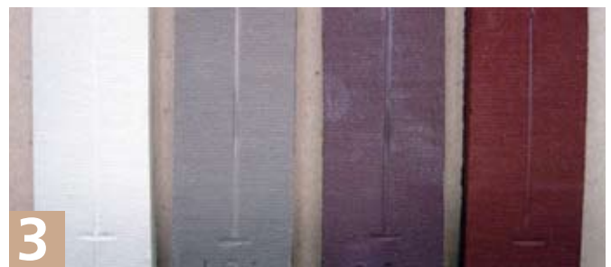
3 Four test bars with a measured and marked 10 cm line.
