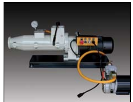
Pugmills blend and homogenize clays. A de-airing vacuum pump removes air from the clay, which in most cases eliminates the need for further wedging. (Photo courtesy Axner Pottery)
