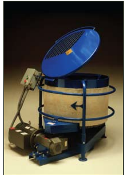
The Soldner mixer is an example of a vertical shaft mixer. This mixer uses a concrete tub that carries clay through stationary bars that blend the clay as it moves through. (Photo courtesy Muddy Elbow Mfg.)
