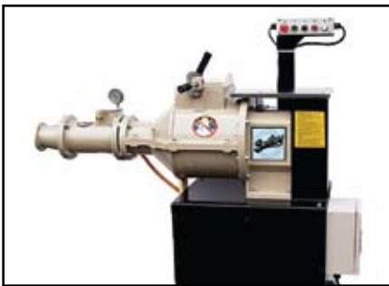
Some mixer/pugmills operate in each mode independently, and many models have optional de-airing available for ready-to-use clay. (Photo courtesy Bailey Pottery Equipment)
