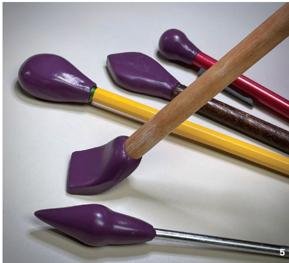
4 Shape the soft silicone onto the stick base and squeeze it tight so it grips on well. 5 You can make any shape you need; thinner silicone will be more flexible. 6 These tools work very well to smooth clay in hard-to-reach places.
