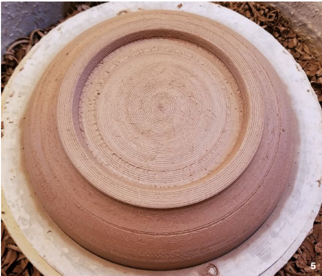
Trim the extra clay until even, while being mindful of the outside surface texture. I use a serrated rib to create texture when done.
