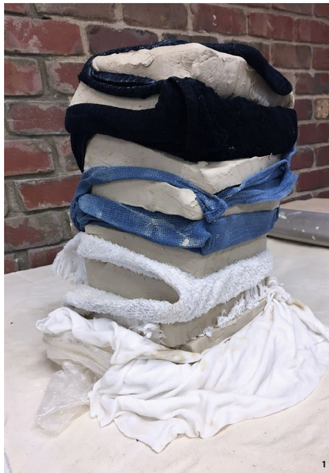
To reclaim dry clay, soak several towels in water, wring them fairly dry, then fold them around 1-inch slices of clay. Wrap the entire set in plastic and allow it sit for a day or two.
