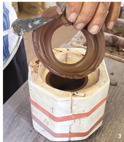
3 Trim the reservoir away, then allow the piece to firm up until it pulls away from the mold.
