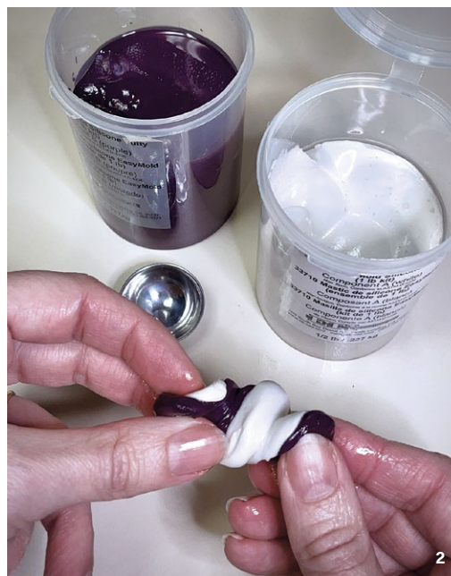
1 Examples of common things that work well as a stick base. 2 Measure and mix equal parts of the two silicone putty ingredients. 3 Roll the mixed putty into a smooth ball to eliminate cracks in the silicone.
