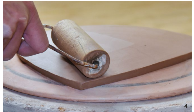
Gently compress the slab with a wooden roller to the curve of the mold.
