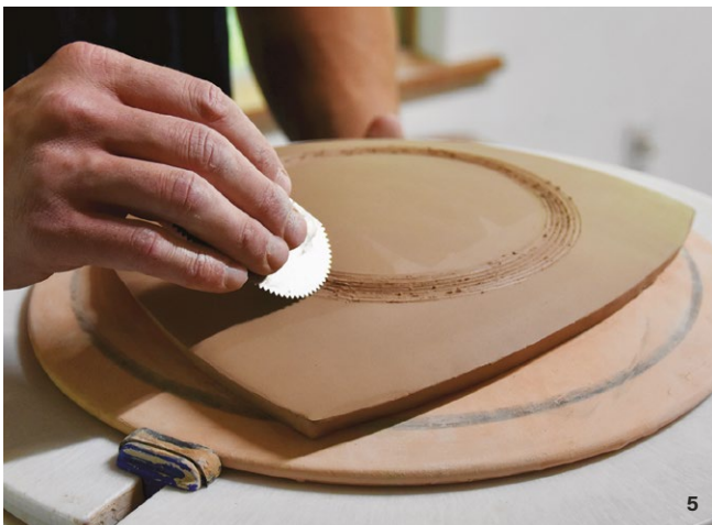
Score the back of the slab in the approximate area where the foot ring will be attached.
