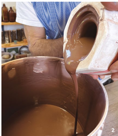
2 Drain the mold and leave it upside down for approximately 10-15 minutes.
