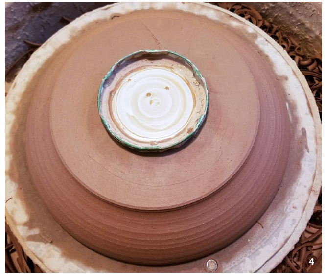
Center the plate. I tap to center and use an old jar lid to hold the plate down.
