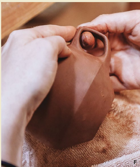
A Maya Rumsey's sketchbook. B Throw the body of the mug. C Pull a handle from a lug of clay, then curve it into the desired shape and set aside to reach soft leather hard. D When the mug reaches leather hard, trim a foot ring into the bottom of the form. E Cut the handle to length, widen the ends, score the attachment areas, apply slip, and attach. F Adjust the angle of the handle to the desired contour. G Sketch surface design motifs using a pencil.
