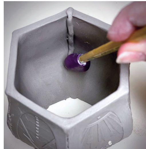
4 Shape the soft silicone onto the stick base and squeeze it tight so it grips on well. 5 You can make any shape you need; thinner silicone will be more flexible. 6 These tools work very well to smooth clay in hard-to-reach places.
