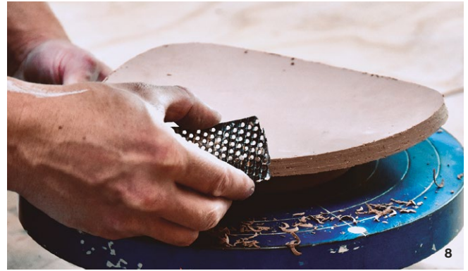
With a metal rasp, do a final shaping of the form. Soften hard edges using a soft rubber rib.
