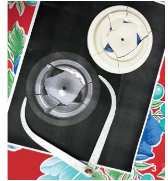
1 Photo of broken teapot lid. 2 The lid taped back together. 3 Enlarged photocopy of the underside of lid being measured with calipers (the broken lid is also included in photo for comparison).
