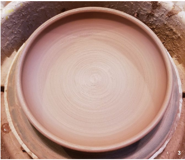
Make sure the inside of the pasta plate is smooth and compressed before taking it off the wheel.
