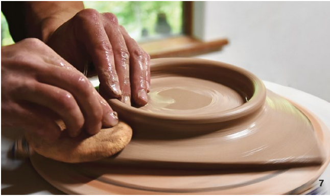
Using a light amount of water, blend the clay of the foot ring into the slab.
