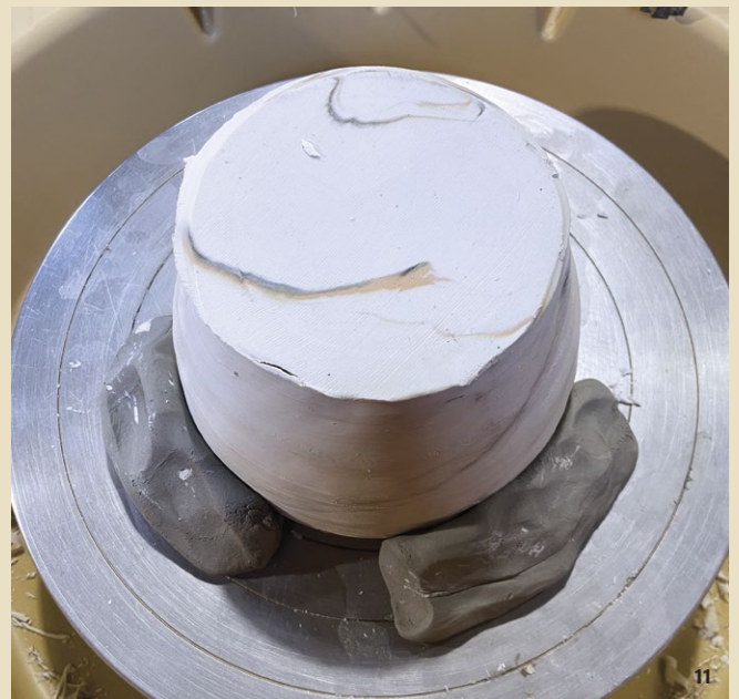
9 Shinro Yamamoto trimming a nerikomi chawan (Japanese tea bowl). 10-13 The leather-hard work is trimmed alternately on the front and back. After bisque firing, burnish the whole surface and fire to temperature. 15, 16 Yamamoto's small anagama kiln. 17, 18 Nerikomi chawan (alternate views), 5½ in. (13 cm) in diameter, porcelain, fired to cone 7, 2023.
