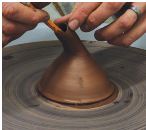
6. Throw a hollow, bottomless cone shape for the spout, then curve it with a pencil.
