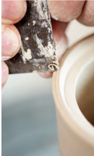
10. Trim an angle into the rim and refine the gallery with a rib.
