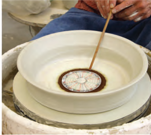
2. Place a dividing web in the center of the open form, and make marks dividing the baking dish into quarters.
