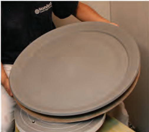
16. Flip the plate back onto a clean, dry bat, and always transport it carefully to avoid warping and cracking.
