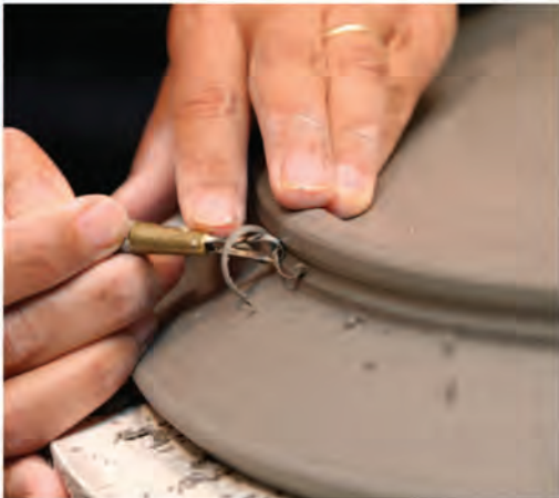
15. If you plan to hang the plate on the wall, carve a deep groove into the outside of the foot ring.
