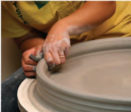
8. Pull up the wall using the index finger on the inside and a sponge and knuckles on the outside.
