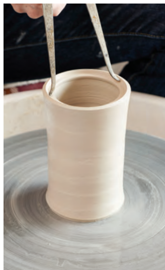
3. Measure the width of the jar's gallery with calipers.
