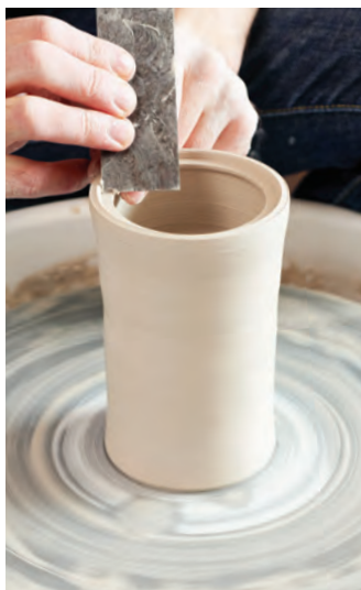
2. Throw the gallery by pressing a steel rib into the inside of the wall.
