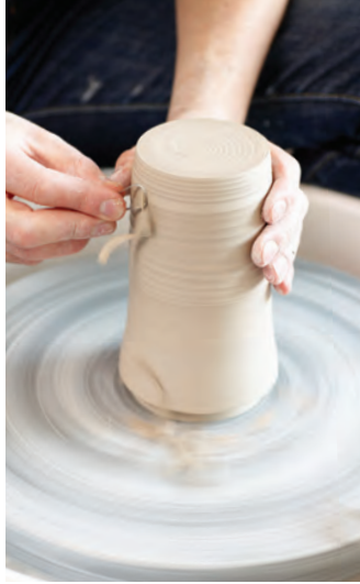
7. Trim the wall of the leather-hard jar using a ribbon trimming tool.
