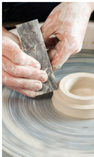
6. Remove excess clay from the lid and refine the lid's flange.
