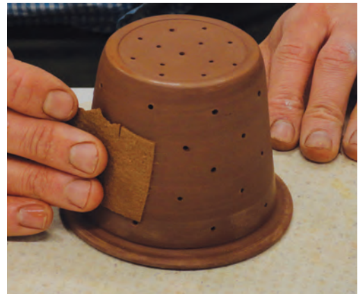
9. Use a needle tool to create holes in the infuser, and smooth the clay with a chamois.
