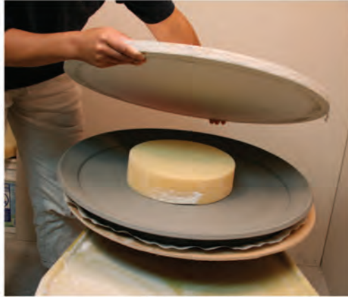
10. Place a foam sheet onto the center of the plate for support while flipping it over.
