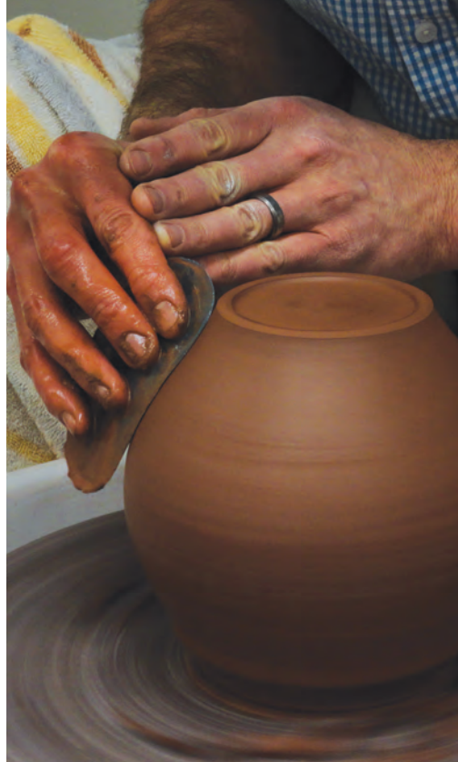
7. Trim the bottom of the teapot body, and compress and smooth the surface with a rib.
