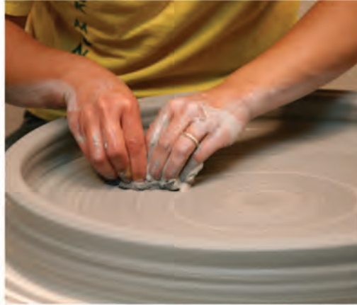
7. Flatten the bottom moving your hands from the center to the edge and back again.
