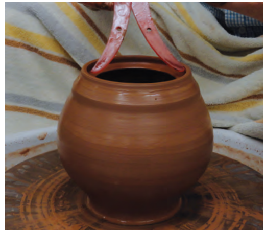
2. Compress, refine, and smooth the shape, and measure the gallery for the infuser.
