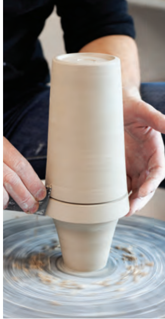
14. Align the lid and jar and trim the walls using a steel kidney.
