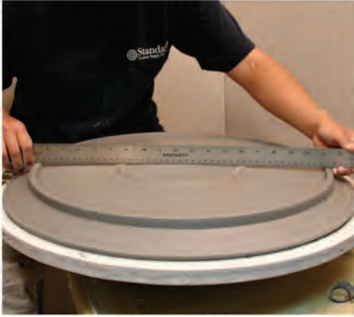
14. Use a ruler or a level to check that the second foot ring is not taller than the outer ring.
