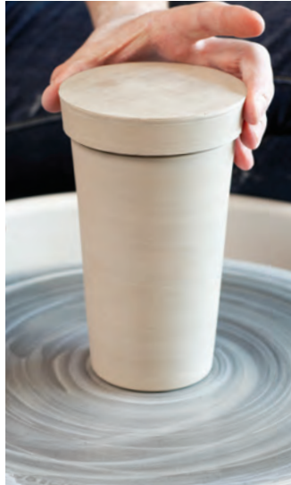
11. Place the lid onto the jar and assess the fit of the rim and flange.
