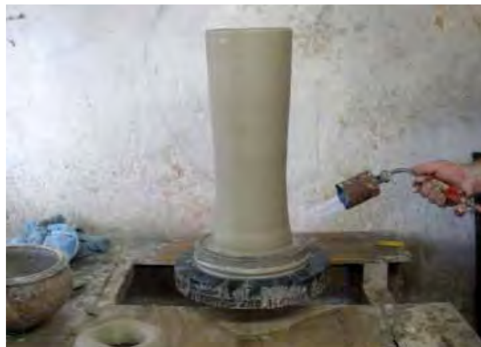
6 Drying the jug base to be firm enough to support the next section.
