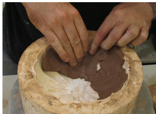
4. Decorative pressings laid into the form mold. Intentional gaps are filled from behind to create depth.
