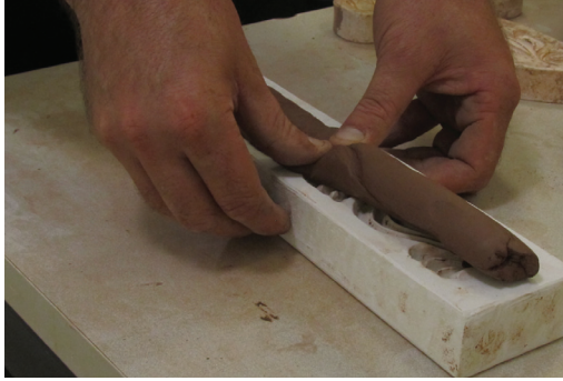
5. A coil is pressed into the decorative mold providing an ornamental strip to coil build with.
