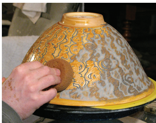
8. Use a sponge to wipe off any black slip that is not in the etched lines.
