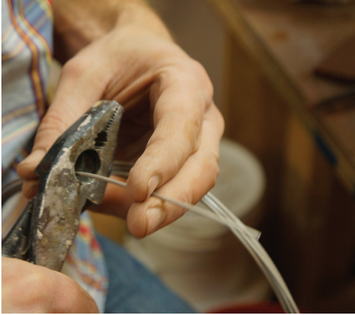
9. Cut nichrome wire to length with wire cutters.
