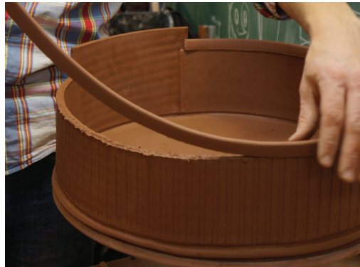
7. Extruded trim pieces are added to finish the rim.
