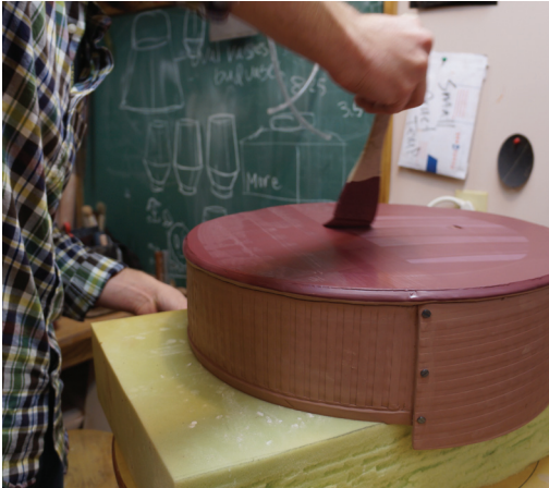
11. Broad strokes of terra sigillata are applied using a hake brush.
