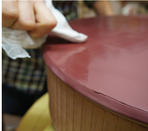
12. Just as the surface sheen has disappeared, burnish it with plastic stretched over a thumb or finger.
