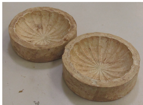
2. A form mold can be used to make an open or closed form.
