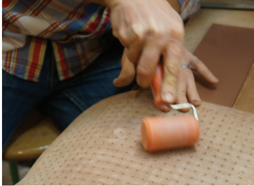
1. A plastic textured mat and a brayer are used to develop the surface of slabs.
