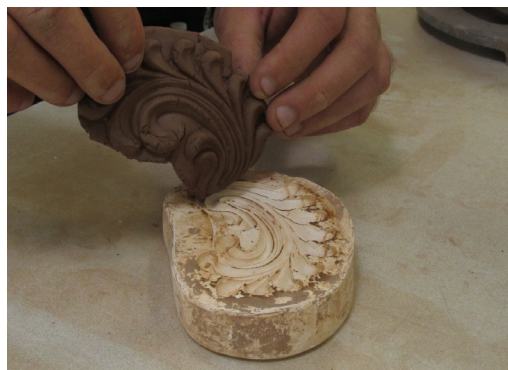
3. Clay pressed into a decorative mold.
