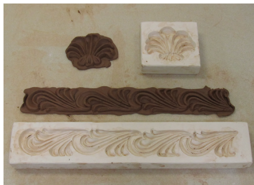
1. Decorative molds and examples of ornamental patties and strips.
