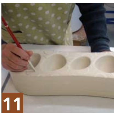
11 Filling the incised lines with a colored slip
