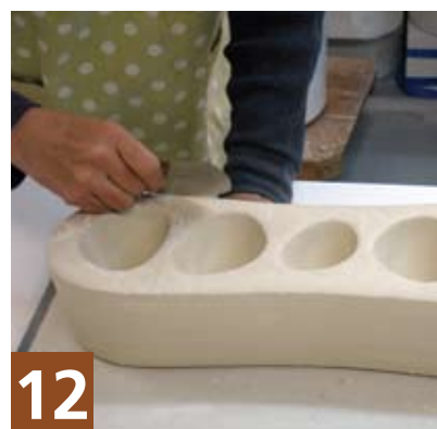
12 Scraping excess slip flush to the surface.
