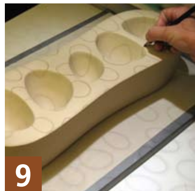
9 Tracing a pattern on the surface using prism projector.
