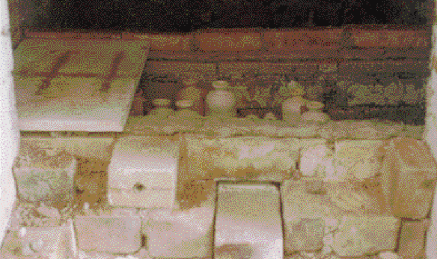
Fig. 4-6. This test kiln was built within the author's downdraft soda kiln. Low brick walls form the front and back walls of a small chamber. Kiln shelves and ceramic fiber are used to make the flat roof. There is provision for an oxygen probe to be inserted through the front wall.
