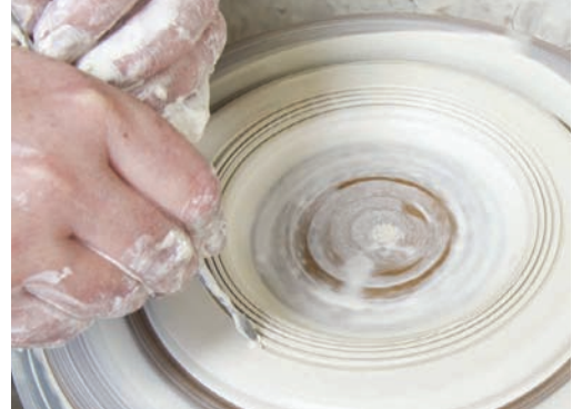
6. Use the shaped end of a sculptor's tool to create a continuous groove on the ring.
