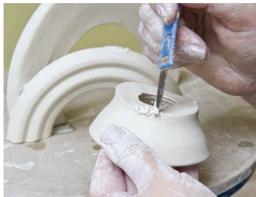
17. Thoroughly score each surface before joining, the same way as you would join a handle to a mug or jug.
