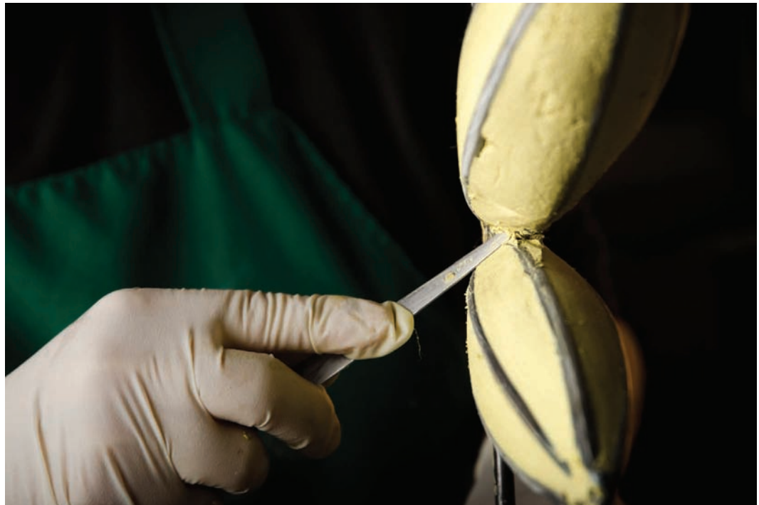
5. Using a fettling knife to smooth the surface of the Egyptian paste between the metal supports and clean excess paste from the supports.
