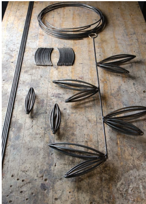
1. Welded \frac{1}{4} -inch steel rods form the frameworks for the sculptures ready for the Egyptian paste to be added.
