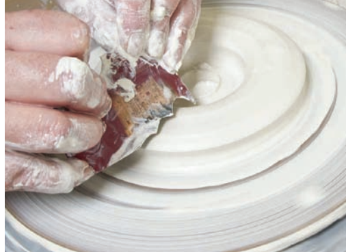
5. Use a flexible, grooved rib (or notched credit card) to contour a thrown ring.
