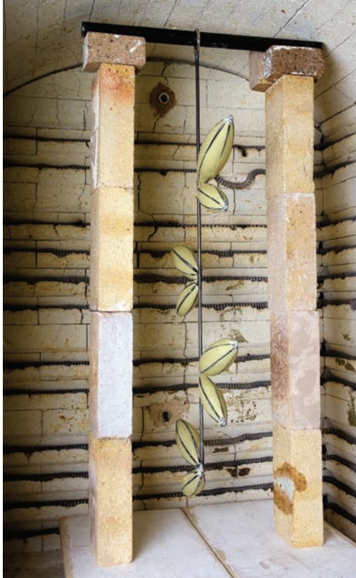
6. Loading the 42-inch tall hanging Wisp structure into the kiln, supported by hard bricks and a black steel pipe.
