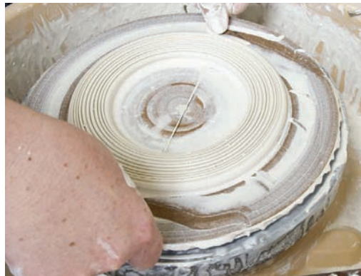
7. Cut a section from the ring with a wire tool held taut against the bat.
