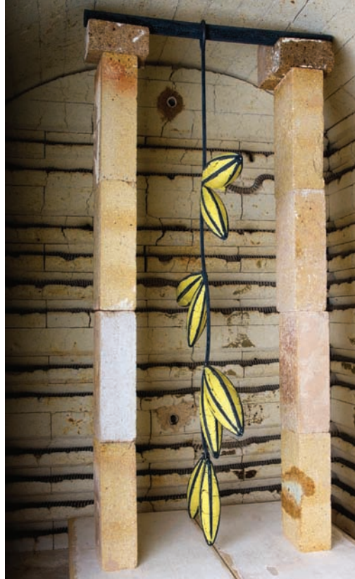
7. After the firing, the metal has serpentine curves due to the action of the heat and weight of the pods.
