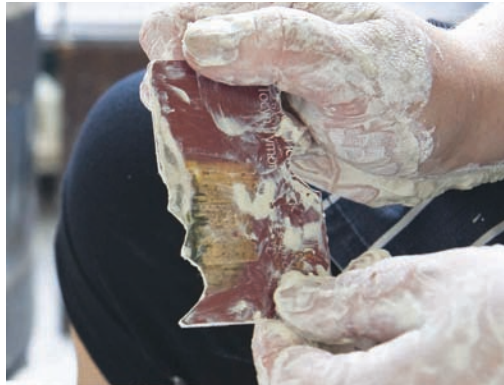
4. This flexible rib with cut grooves is made from an old credit card.
