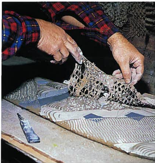
Coloured slips and cloth textures are applied to slabs.
