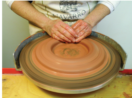
She then throws a ring without a bottom to form the walls of the baking dish.
