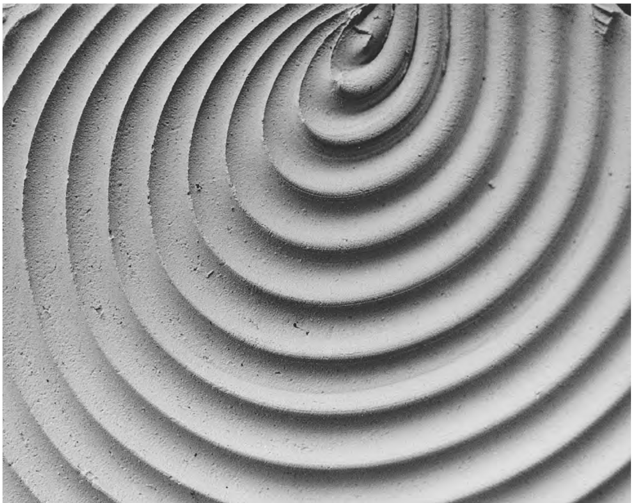
Fig. 9.6 Shell-like pattern produced from a cutting cord or wire.
