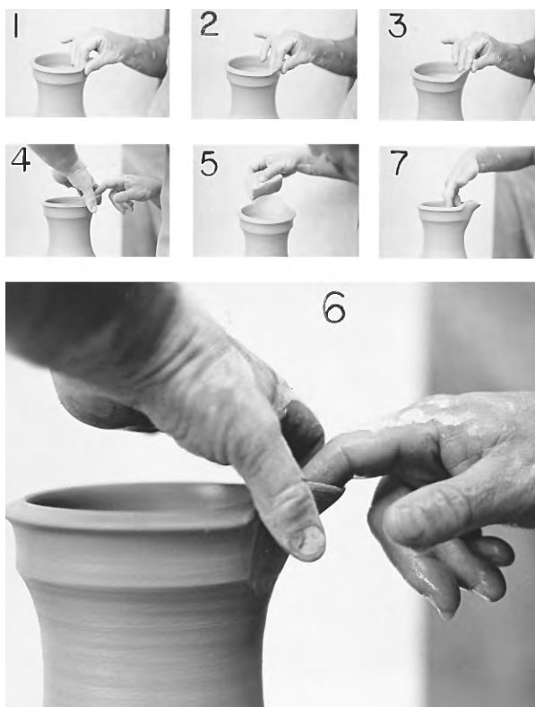
Fig. 9.11 Pulling a spout: 1 - 3. Pinching out the thickened lip to thin the edge; 4. Starting a pouring lip; 5. Sponging the curve of the lip; 6. Pulling the pouring lip; 7. Easing out the throat to give a good inner pouring surface.
