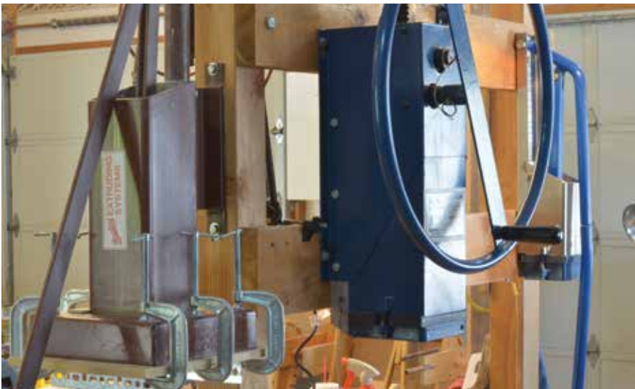
Extruders mounted on 4×4 posts and 2×4s. Follow the manufacturers instructions carefully when mounting an extruder in your studio.
