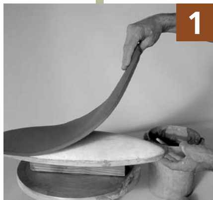
Place a slab over the mold.
