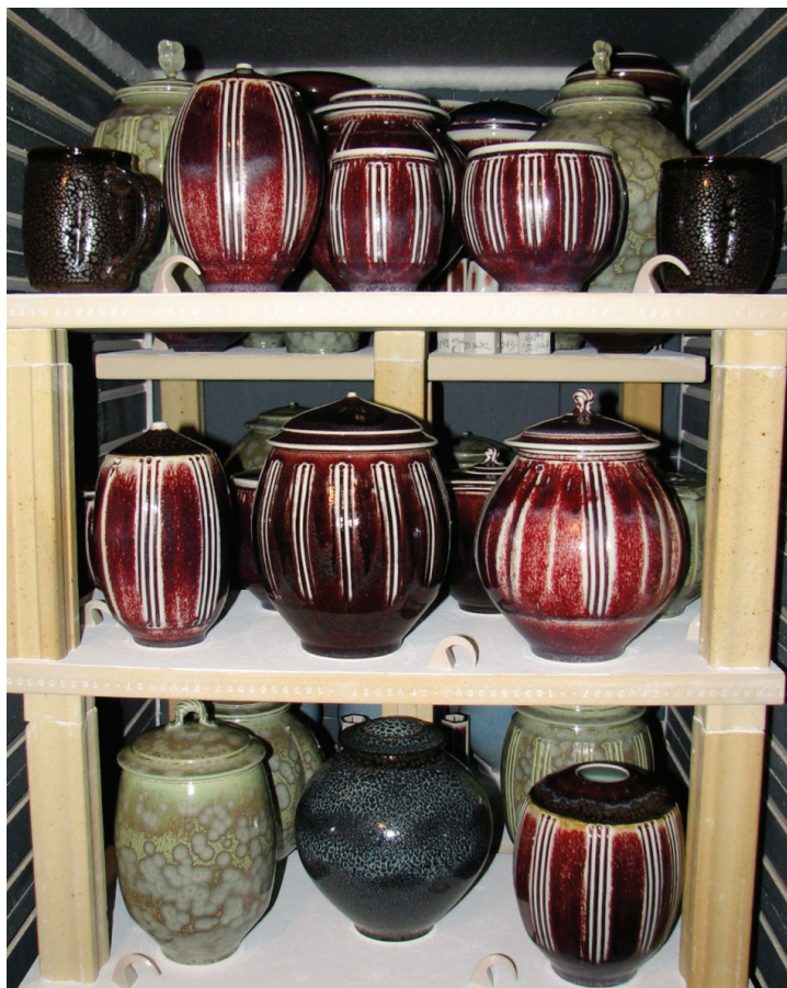
This image shows one of Tom Turner's perfectly even glaze firings from his 12-cubic-foot front-loading electric kiln. Notice the cone placement and how there is no difference between any of the cones. Placing cones all around the firing chamber like this allows you to see if there are hot or cool spots in your kiln. These pieces are glazed with copper red oxblood, oilspot, and non-running zinc crystal glazes developed by Turner. 2012. Photo by Steve Mann
