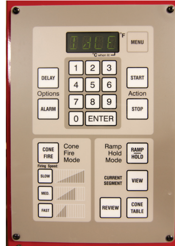
An example of a control panel on a computerized kiln. Though computerized kilns may take some of the know how out of the firing procedure, they do make firings less time consuming and more energy efficient.
