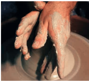
7 With continuing side pressure to prevent mushrooming, press clay back down.
