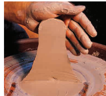
6 Cross section showing maximum rise. Heel of thumb poised to press clay down.
