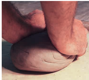
2 Lean into the lump, smearing the lower portion against the wedging table.
