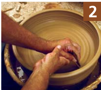
2 Throw a low wide cylinder and cut out the bottom.
