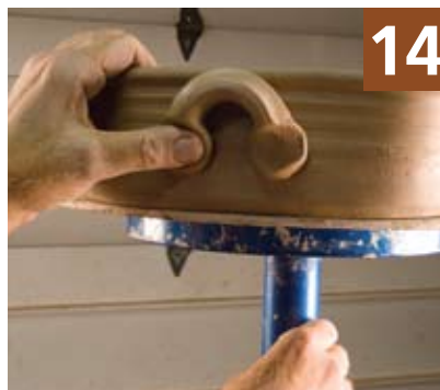
14 Attach pulled handles using water or slip.
