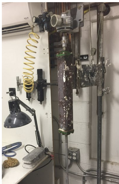
Left: A variable speed high-sheer mixer made by the author using off-the-shelf parts. Middle: The spray system and washout tub. Right: A typical airline drop with filters.
