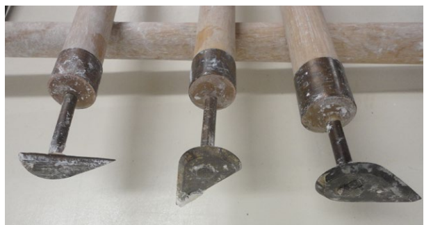
A selection of specially made turning tools in various profiles.
