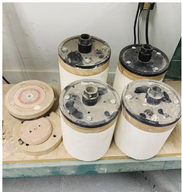
Top: A system using a standard lathe faceplate to secure RenShape. Middle: Lathe with special bucket head and mandrel. Above: Solid plaster cylinders ready for turning.
