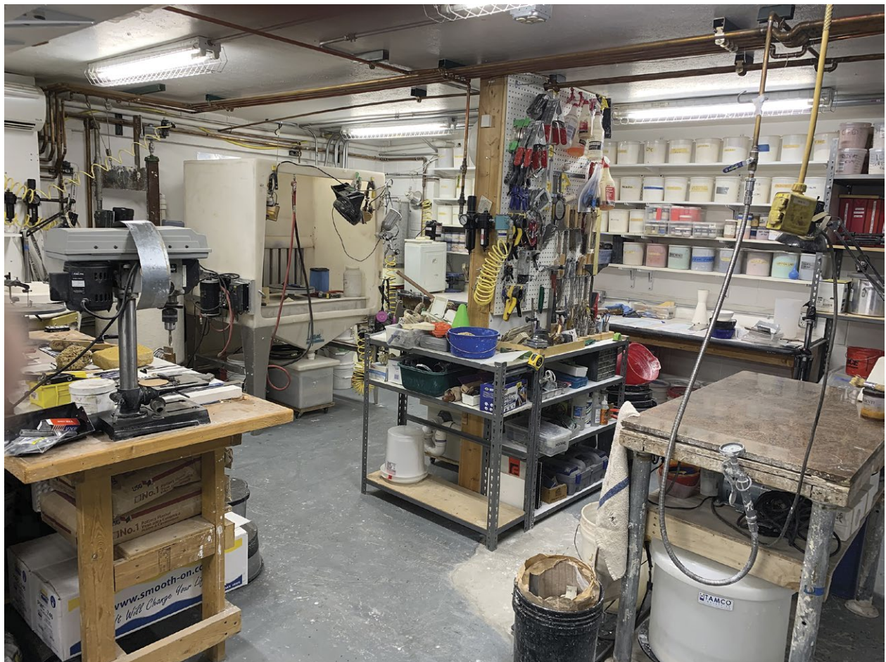
Part of the author's work space, with work stations for turning plaster, mold making, and mixing and spraying glaze.
