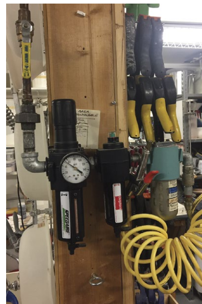
Left: A variable speed high-sheer mixer made by the author using off-the-shelf parts. Middle: The spray system and washout tub. Right: A typical airline drop with filters.
