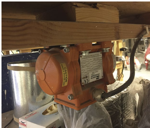
A small electric vibrator, mounted under the author's table.
