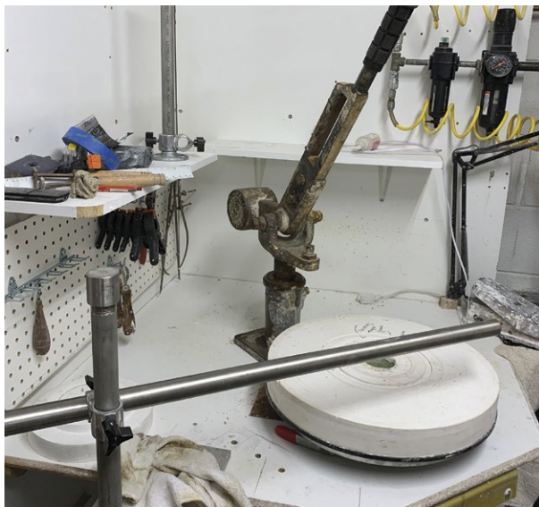
A potter's wheel adapted for vertical turning and jiggering plaster forms.
