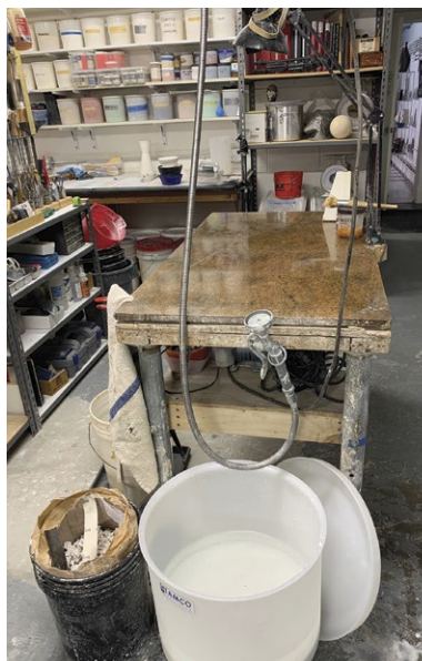
Left: A variable speed high-sheer mixer made by the author using off-the-shelf parts. Middle: The spray system and washout tub. Right: A typical airline drop with filters.
