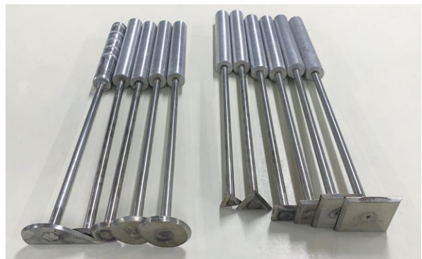
Long-handled plaster turning tools for use with a belly stick.
