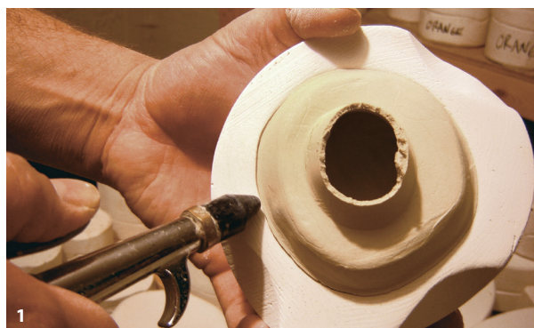
1 Use compressed air to separate the mold and to release the thin clay form without distorting it.
