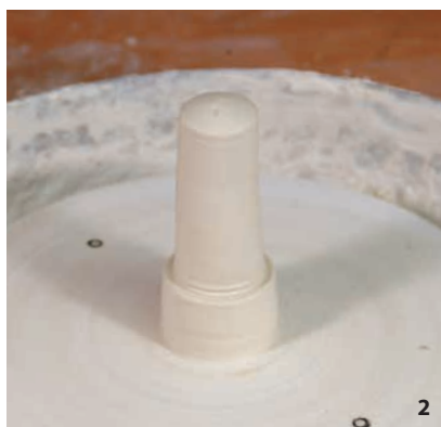
Collar in to close off the top of a thrown cylinder, then use a rib to define the collar where the peephole plug meets the outside of the kiln.
