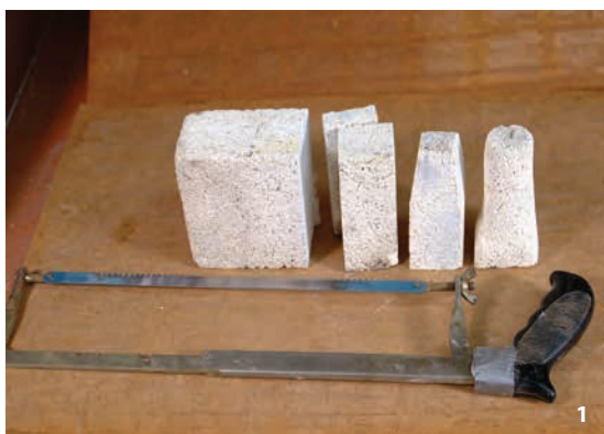
Soft brick cut in half then in fourths, hack saw to taper cut the four corners and finished with coarse sand paper. The one on the far right is finished and ready to use.
