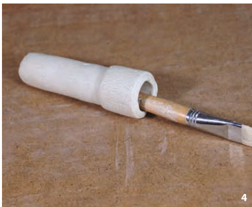
Roll a wooden rod inside the cylinder to shape the handbuilt peephole plug.
