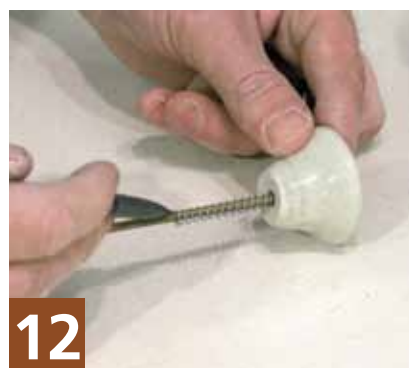
12 After inserting a scrap piece of rod and a spring into the knob, make a mark where the spring ends.
