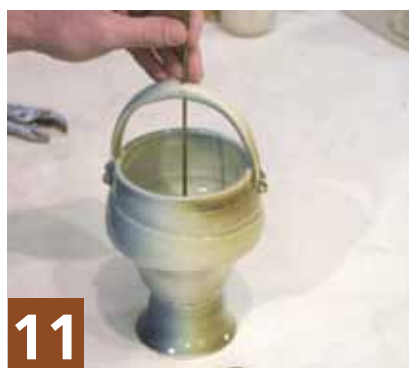
11 Pull the rod up and check that the plug fits securely into the opening. Set the pancaker aside.
