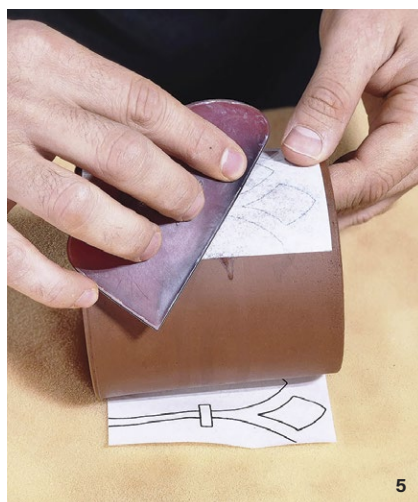
5 Compress the transfer paper onto the mug with a soft rubber rib.
