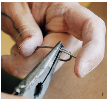
1 Using needle-nose pliers, twist wire into an arced shape and doubled-up loops.
