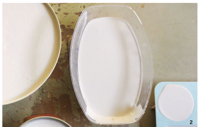
1 Set up your space with plaster, water, vessels, and a selection of tools. 2 After pouring plaster into your vessels, gently agitate to release trapped air bubbles before letting the plaster cure.
