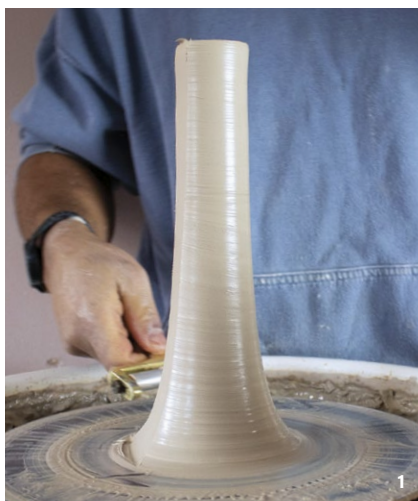
1 Pull a tall, skinny cylinder. Make vertical facets from the wheel up to the rim.
