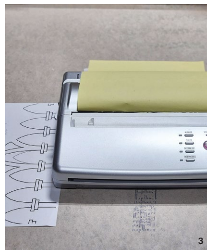
3 Use a thermal printer to make a transfer with cleaner, crisper lines in the design.
