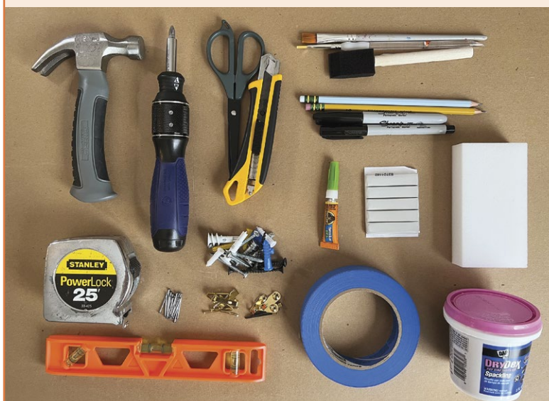
Gather the tools you find to be useful for installing your work and keep them together. Shown here (clockwise from top left): a small hammer, ratcheting screwdriver with Phillips-head bit, scissors, utility knife, assorted brushes, pencils, permanent markers, super glue, poster tack, melamine sponge, spackle, painter's tape, assorted hardware, level, and tape measure.
