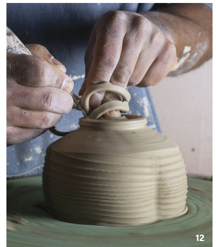
Carve the inside of foot, and then refine the ring and bottom.
