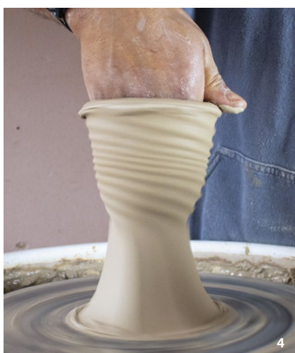
4 Work your hand to the bottom and compress as you drag your fingers up the wall.
