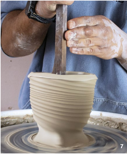
Use a throwing stick to gently open the form wide enough to fit a large rib.
