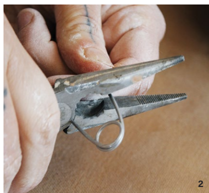
2 Leave at least ½ inch (1.3 cm) of straight wire on each end to insert into the piece.
