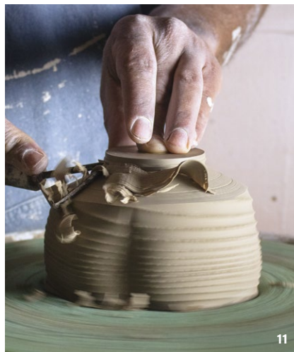
Trim the bulk of clay off the bottom and create the exterior of the foot ring.
