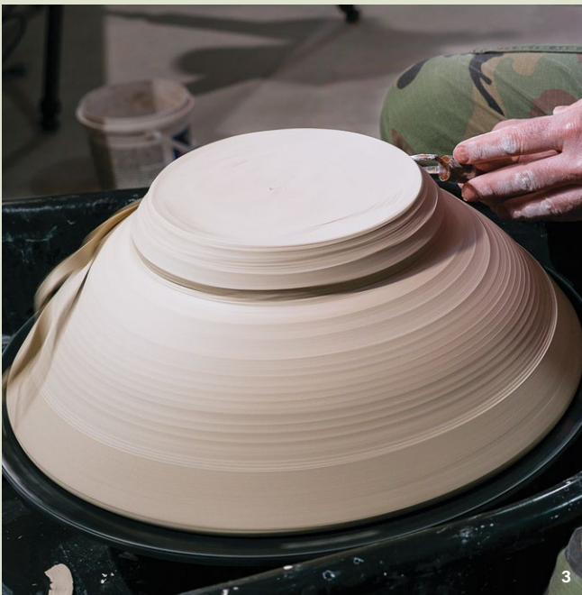
1 Lansing Wagner cutting out the lobster design from a scanned, resized, and printed copy of a drawing. 2 Throw the bowl, using a rib to shape the interior curve and compress the clay. 3 Trim with a loop tool to define the foot on the bowl and remove excess clay from the outside wall. 4 Spray blue slip on the inside and outside of the leather-hard bowl.
