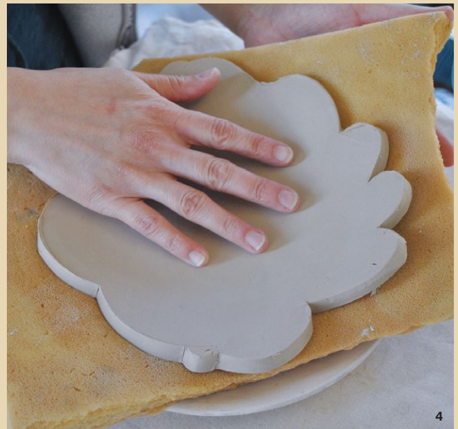
1 Tools used the most: soft rubber rib, stylus, sponge, various brushes, knives, and a bisque mold. 2 Cut away following the outline that was loosely drawn with a rubber-tipped tool beforehand. 3 Place the slab on a piece of foam, then set both on a bisque-mold plate form. 4 Lightly press the slab into the foam to bring the edges up slightly.
